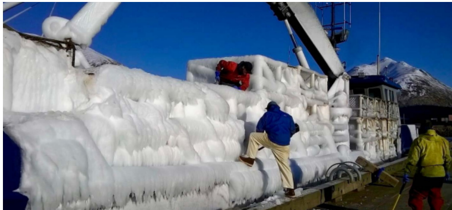
Figure 1: Ice accumulation on Sandra Five , National Transportation Safety Board (2017).
